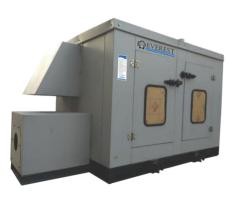
Everest Sound reduction enclosures have been designed for effective noise reduction of blowers placed inside. Everest's economical design provides noise reduction of 12-25 dB(A) bringing down the total noise emitted to safe acceptable limits.
